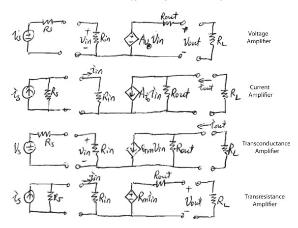
For the above single stage amplifiers (i.e. CS, CD, CG, CE, CC, CB), as we identify their particular function, e.g. current buffer is a type of current amplifier. We can use a *two-port model* for current amplifier to model a CB or CG circuit. Their corresponding  $R_{\rm in}$ ,  $R_{\rm out}$ ,  $A_{\rm io}$  will depend on the circuit (or device parameter), which we can derive based on the *small* signal circuit model of the circuit.
