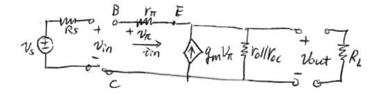
Cast this into two port voltage amplifier model
