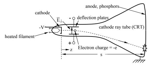
Figure 5.1.1 Cathode ray tube.
