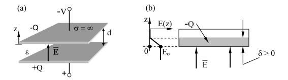
Figure 5.2.1 Charge distribution within conducting capacitor plates.
