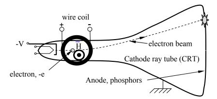
Figure 5.1.2 Magnetic deflection of electrons in a cathode ray tube.
