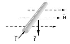
Figure 5.2.2 Magnetic force on a current-carrying wire.
