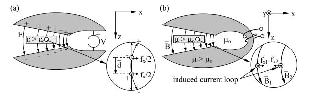
Figure 5.3.1 Kelvin polarization and magnetization forces on materials.
