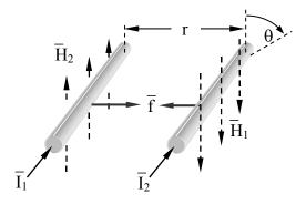
Figure 5.2.3 Magnetic forces attracting parallel currents.
