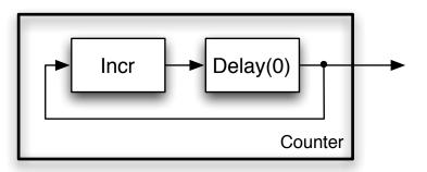
Figure 4.7 Counter made with feedback and serial combination of an incrementer and a delay.
