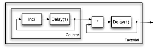
Figure 4.9 Machine to generate the Factorial sequence.
