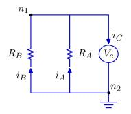
we have a simple circuit with two resistors in parallel. Even though there are a lot of wires being connected together, there are really only two *nodes*: places where multiple components are connected. Let's write down the equations governing this system.
