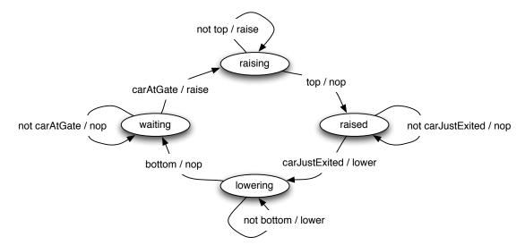
Figure 4.3 State transition diagram for parking gate controller.
