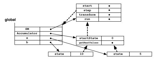
**Figure 4.2** Classes and instances for an Accumulator SM. All of the dots represent procedure objects.
