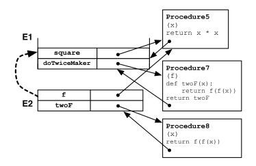
Here is a picture of the environments after the doTwiceMaker returns its value and it is assigned to twoSquare in E1. It is important to see that Procedure8 is the return value of the call to doTwiceMaker and that, because Procedure8 retains a pointer to the environment in which it was defined, we need to keep E2 around. And it is E2 that remembers which procedure (via its binding for f) is going to be applied twice.
