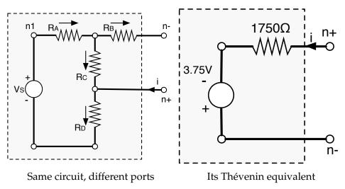
Note also that the top lead is marked  $n_-$  and the bottom one  $n_+$ . If we solve, using the same values for the resistors and voltage source as before, we find that  $V_{th} = -3.75V$  and  $R_{th} = 1750\Omega$ . We show the Thévenin equivalent circuit next to the original. We've changed the polarity of the voltage source and made it 3.75V (instead of having the + terminal at the top and a voltage of -3.75), but that's just a matter of drawing.
