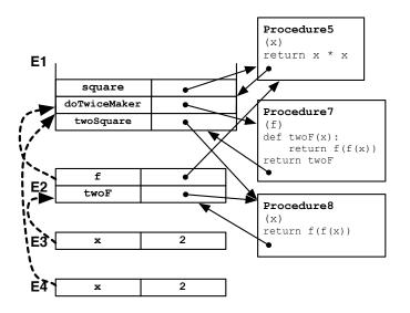
Evaluating the body of Procedure5 in E4 yields 4. We will repeat this process to evaluate the outer application of f, in f(f(x)), now with argument 4, and end with result 16.
