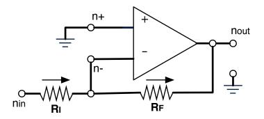
The difference is that the + terminal of the op-amp is connected to ground, and the we're thinking of the path through the resistors as the terminal of the resulting circuit. Let's figure out the relationship between  $v_{in}$  and  $v_{out}$  for this one. The circuit constraints tell us that
