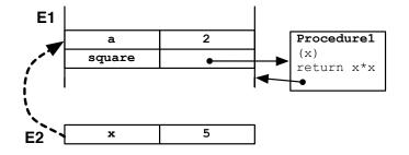
The dotted line between E2 and E1 is intended to indicate that E1 is the *parent environment* of E2.
