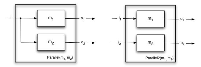
Figure 4.5 Parallel and Parallel2 compositions of state machines.
