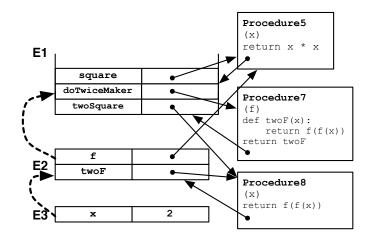
Next, we evaluate the body of Procedure8, which is return f(f(x)) in E3. Let's just consider evaluating the inner expression f(x) in E3. We evaluate f in E3 and get Procedure5, and evaluate x and get 2. Now, we make a new binding environment, E4, to bind the formal parameter of Procedure5 to 2. Because Procedure5 has a stored pointer to E1, E4's parent is E1, as shown here:
