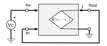
Note that we have connected a wire from the output,  $n_{out}$ , to the negative input,  $n_{-}$ , and so those constitute one node with a single voltage, which we call  $v_{out}$ . We can write down the equations:
