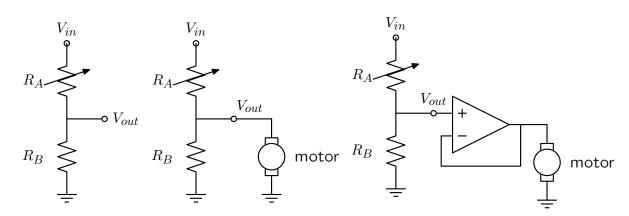
**Figure 1.3** Voltage dividers: A. Resistor divider. B. Connected to a motor, in a way that *breaks* the abstraction from part A. C. Connected to a motor, with a buffer.
