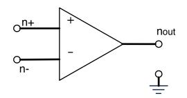
The simplified behavioral model is that the op-amp adjusts  $v_{out}$  in order to try to maintain the constraint that  $v_+ \approx v_-$  and that no current flows in to  $n_+$  or  $n_-$ . In what follows we will assume that the op-amp enforces  $v_+ = v_-$ .
