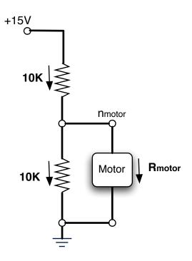
But what will the voltage  $v_{motor}$  end up being? It all depends on the resistance of the motor. If the motor is offering little resistance, say 100 $\Omega$ , then the voltage  $v_{motor}$  will be very close to 0.<sup>43</sup> So, this is not an effective solution to the problem of supplying 7.5V to the motor.
