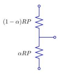
By connecting a potentiometer as shown below we can create a device that converts a into a voltage Vo. **All voltages are measured relative to ground**.
