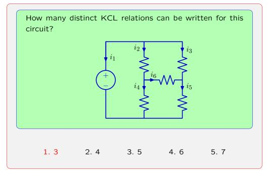
The number of independent KCL equations is one less than the number of nodes.
