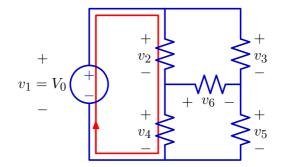
Example:  $-v_1 + v_2 + v_4 = 0$  or equivalently  $v_1 = v_2 + v_4$ .
