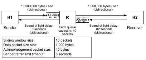
Figure 1: Ben's network configuration, with initial network parameters.
