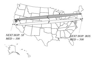
Figure 8: MED's are useful in many situations, e.g., if C is a transit customer of P, to ensure that cross-country packets to C traverse P's (rather than C's wide-area network). However, if C and P are in a peering relationship, MED may (and often will) be ignored. In this example, the MED for  $D_S F$  is set to 100 at the SF exchange point, and 500 in Boston, so P can do the right thing if it wants to.
