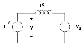
Figure 3: Inverter Connected to Power System
