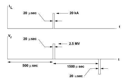
Figure 2: Shorted end current and matched end voltage
