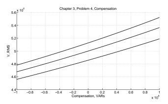
Figure 4: Receiving End Voltage
