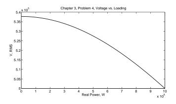
Figure 3: Receiving End Voltage
