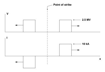
Figure 1: Pulses at about 40 microseconds
