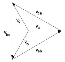
Figure 6: Three-Phase Voltages
