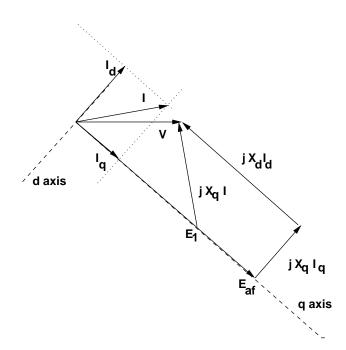
Figure 6: Vector Diagrem for Salient Pole Machine
