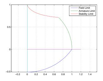
Figure 7: Capability Curve for Salient Pole Machine (per-unit)
