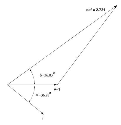
Figure 1: Voltage Vector Diagram of part a
