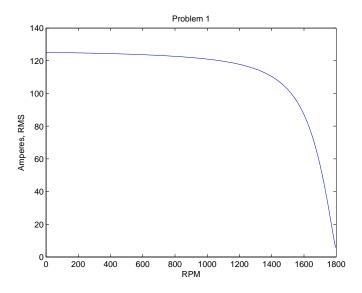
Figure 3: Induction Motor Current vs. Speed
