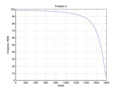
Figure 6: Induction Motor Current vs. Speed
