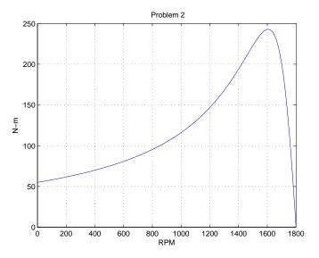
Figure 5: Induction Motor Torque vs. Speed
