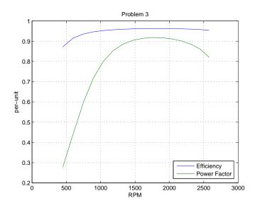
Figure 11: Volts per Hz. Efficiency and Power Factor vs. Speed
