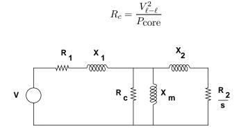
Figure 1: Induction Motor Equivalent Circuit
