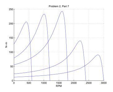
Figure 9: Torque vs. Speed, Volts/Hz Control
