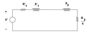
Figure 2: Induction Motor Equivalent Circuit
