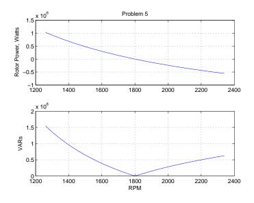
Figure 13: Real and Reactive Power into Slip Rings of DFM
