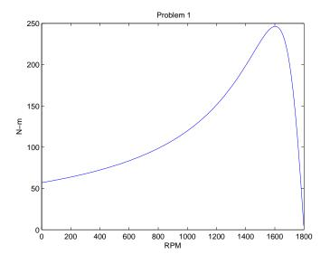
Figure 4: Induction Motor Torque vs. Speed
