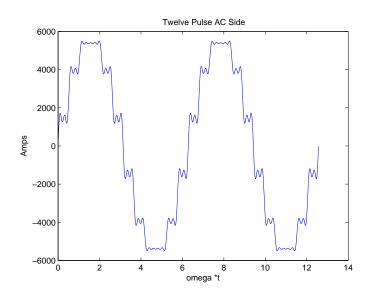
Figure 2: Reconstructed AC Waveform: Twelve Pulse
