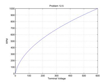
Figure 3: Speed vs. Voltage for Series Motor
