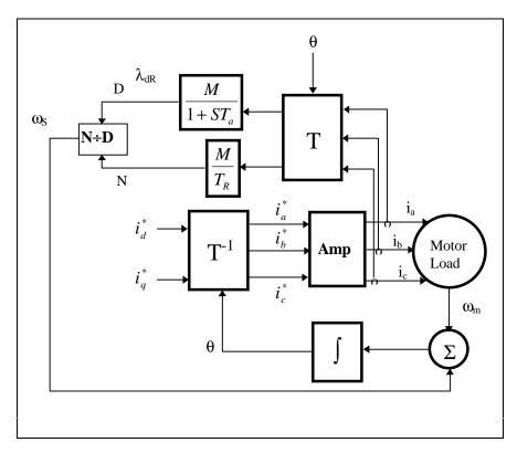
Figure 16: Field Oriented Controller
