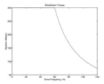
Figure 15: Idealized Torque Capability Curve: Zero Stator Resistance
