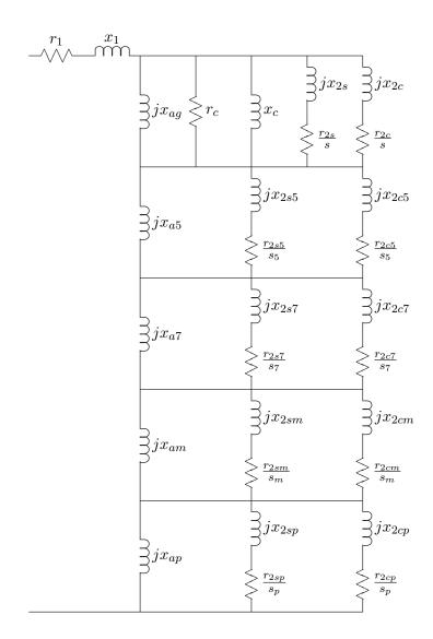
Figure 17: Extended Equivalent Circuit
