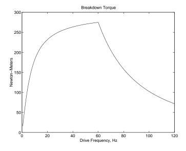
Figure 14: Torque-Capability Curve For An Induction Motor
