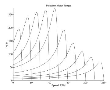
Figure 10: Induction Machine Torque-Speed Curves
