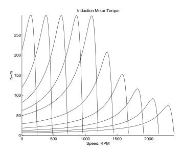
Figure 13: Idealized Torque-Speed Curves: Zero Stator Resistance
