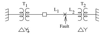
Figure 14: One-Line Diagram For Example Fault
