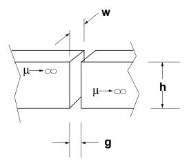
Figure 3: Gap between magnetic elements
