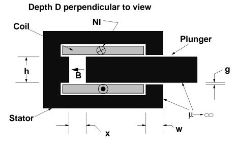
Figure 6: Cross-Section of Solenoid Actuator
