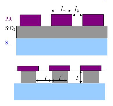
b) Use Fig. 10-23 in Plummer (p. 28 in "dry etch" class notes) to determine the minimum thickness of photoresist applied in terms of l, if you are going to be using an etchant of 40% H<sub>2</sub> in CF<sub>4</sub> +H<sub>2</sub>.
