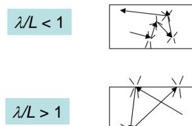
Flow is viscous; p > 1 mT Deposited species "thermalized"; Growth is from all directions, good step coverage
