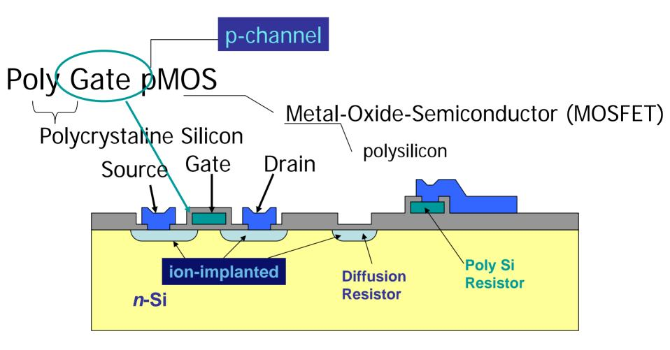
Field oxide grown in steam, gate oxide made by CVD *p*-regions ion-implanted, AI sputter deposited or evaporated
