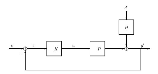
Figure 17.7: Example of a unity feedback system.
