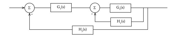
To obtain the forward path of the major loop, we just overlay plots of  $G_1(s)G_2(s)$  and  $G_1(s) \cdot \frac{1}{H_1(s)}$ . The forward path is the lower of the two curves at all frequencies
