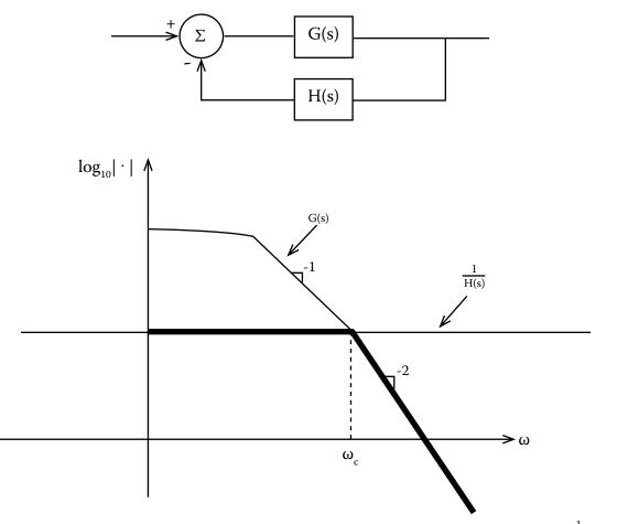
The trick for graphing the closed-loop response for the system was to overlay G(s) and  $\frac{1}{H(s)}$  , and then
