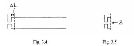
Thus the problem can be solved approximately by finding the length  $\Delta \ell$  for which the impedance Z looking into the short tube in Fig. 3.5 is infinity at each of the original two lowest natural frequencies of the tube. Note that this short tube is effectively a Helmholtz resonator.
