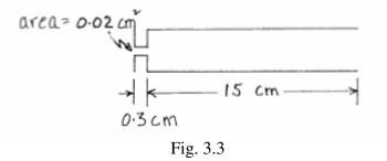
The natural frequencies are the frequencies for which the sum of the impedances looking to the left  $(Z_L)$  and to the right  $(Z_R)$  at the left end (as shown) is equal to zero, i.e.,
