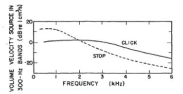
Figure 2.49 The solid line gives the estimated spectrum amplitude (in 300-Hz bands) of the transient source that occurs at the abrupt release of a click, as in figure 2.48. An enclosed volume of air equal to  $1.0 \text{ cm}^3$  is assumed, with a negative pressure of  $100 \text{ cm} \text{ H}_2\text{O}$  within this volume at the instant of release. The calculated transient for a release of a pulmonic alveolar or labial stop consonant is shown for comparison, from figure 2.47 (dashed line).
