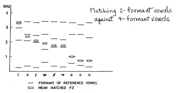
Figure 4.34 The horizontal lines give the first four formant frequencies of a set of Swedish vowels used in a matching experiment. The boxes show the mean frequency of the second formant (F2') of a two-formant stimulus that gave a best match to the full vowel. F1 of the two-formant matching stimulus was set to F1 of the vowel. (From Carlson et al., 1970.)
