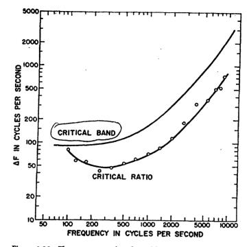
**Figure 4.30** The upper curve plots the width  $\Delta F$  of the critical band as a function of the center frequency of the band, as measured in masking experiments that manipulate the bandwidth of the masker. The lower curve gives the bandwidths calculated from the critical ratio, as in figure 4.25. (From Greenwood, 1961a.)
