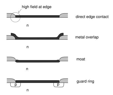
If p guard ring used, must make sure that p-n junction never turns on.
