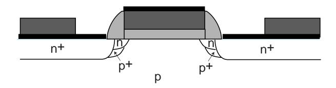
circa~1994  $L \sim 0.15 \ \mu m$   $x_{ox} \sim 60 \ \mathring{A}$   $x_j \sim 0.08 \ \mu m$  $V_{DD} = 2.5 \ V$
