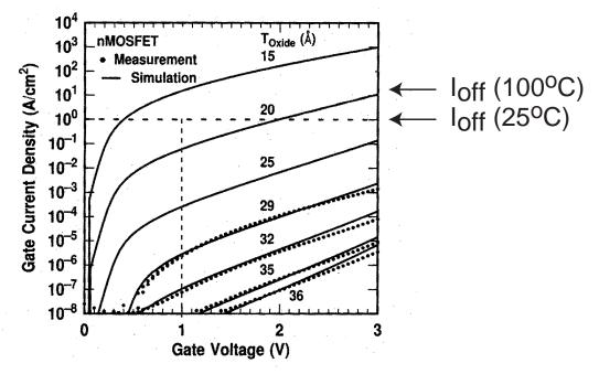
Fig. 2. Measured and simulated  $I_G-V_G$  characteristics under inversion conditions of four nMOSFET's. The dotted line indicates the 1 A/cm<sup>2</sup> limit for leakage current as discussed in the text.
