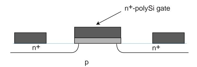
circa~1980  $L \sim 2 \ \mu m$   $x_{ox} \sim 400 \ \mathring{A}$   $x_j \sim 1 \ \mu m$  $V_{DD} = 5 \ V$
