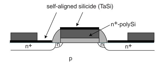
circa~1989  $L \sim 0.4 \ \mu m$   $x_{ox} \sim 125 \ \mathring{A}$   $x_j \sim 0.15 \ \mu m$  $V_{DD} = 3.3 \ V$
