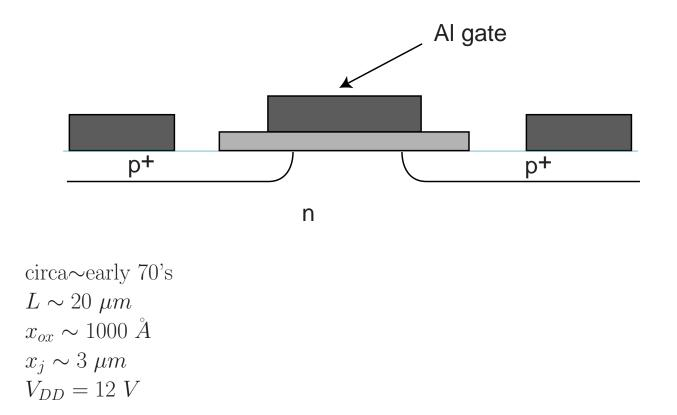
Main point: Na<sup>+</sup> contamination made NMOS devices to have too negative a threshold voltage
