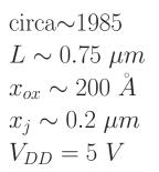
Main point: lightly-doped n-region on drain side reduces electric field there and allows a high  $V_{DD}$  to be used.
