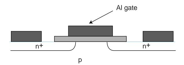
circa~1975  $L \sim 15 \ \mu m$   $x_{ox} \sim 600 \ \mathring{A}$   $x_j \sim 2 \ \mu m$  $V_{DD} = 12 \ V$
