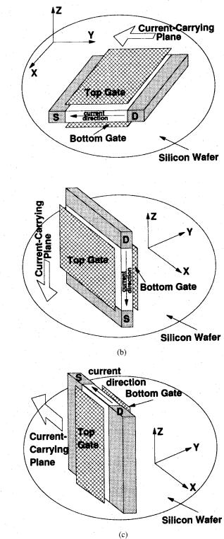
Fig. 29. Three possible orientations of a double-gate MOSFET on a silicon wafer. Examples of devices fabricated are: (a) Colinge *et al.* [54], Tanaka *et al.* [55], (b) Takato *et al.* [56], and (c) Hisamoto *et al.* [57].
