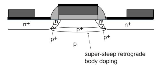
circa~late 90's (manufacturing in early 00's)  $L < 0.1 \ \mu m$   $x_{ox} \sim 30 \ \mathring{A}$   $x_j \sim 0.06 \ \mu m$  $V_{DD} = 0.8 - 1.5 \ V$
