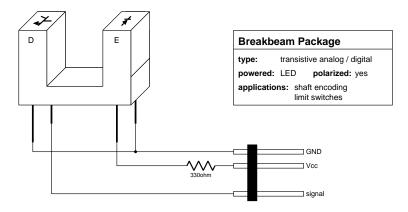
Figure 5.7: Breakbeam sensor package
