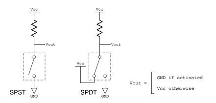
Figure 5.1: Digital Sensor Circuit
