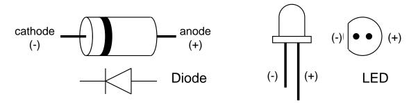
Figure 4.5: Identifying diode leads
