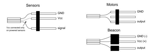
Figure 4.7: 6.270 connector standard
