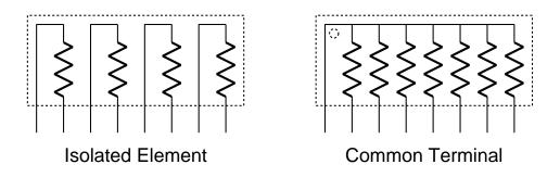
Figure 4.4: Resistor pack internal wiring
