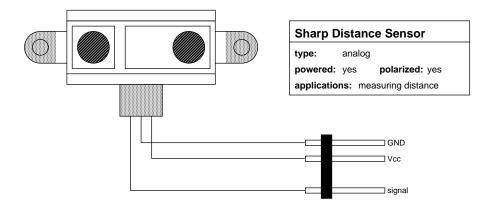
Figure 5.8: Sharp Distance Sensor
