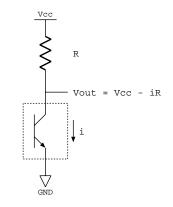
Figure 5.5: Transistive Analog Sensor Circuit
