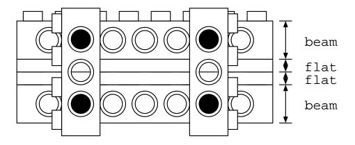
Figure 6.2: A Simple Braced Structure
