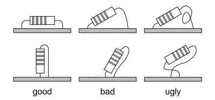
Figure 4.2: Axial component mounting
