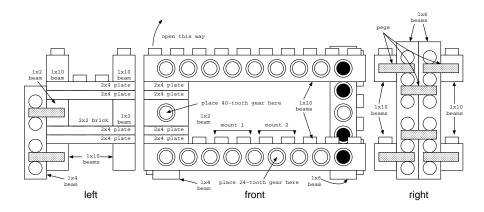
Figure 4.8: Jig for motor assembly
