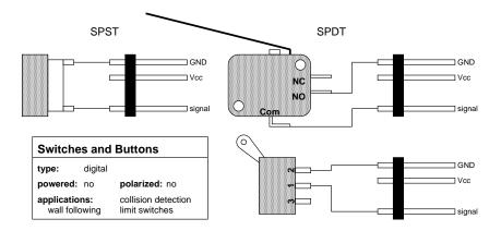
Figure 5.2: Switches and buttons
