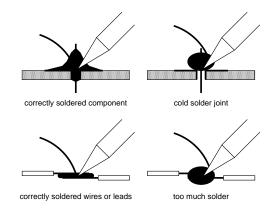
Figure 4.1: Good and bad soldering technique
