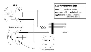
Figure 5.6: LED and Phototransistor
