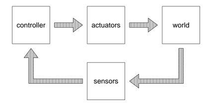
Figure 7.3: Closed loop (feedback) information flow
