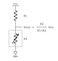
Figure 5.3: Resistive Analog Sensor Circuit
