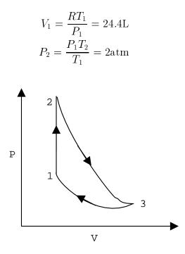
Figure 1: P-V diagram cycle
