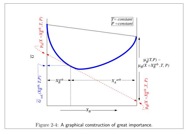
This construction and the equality of chemical potentials results in the common tangent construction between several phases of heterogeneous solution in a binary alloy:
