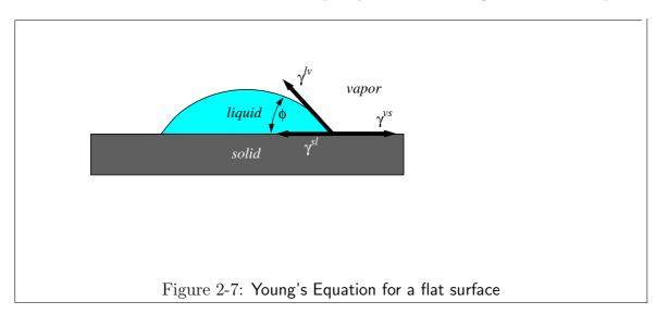
Surface tensions act a force balances and specify the contact angle between two phases:
