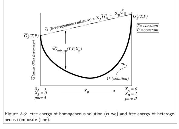
The reduction in free energy at a fixed composition drives systems into solution.
