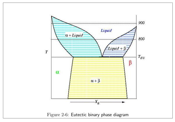
The two phase regions are composed of the limiting compositions on either side of the two-phase region on the phase diagram; the *lever rule* allows us to determine the fractions of each phase.
