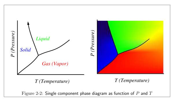
A phase diagram is a map that tells you what phases will be stable at what conditions. You *must* understand and be able to explain how these diagrams follow from plots of free energy curves—this involves using intersections of the free energy curves and the common tangent construction.
