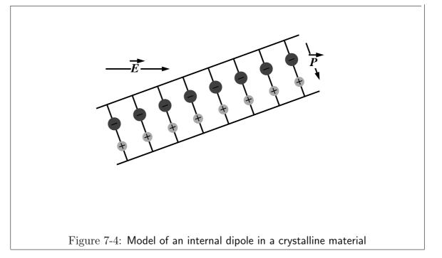
The polarization is not necessarily in the direction of the field. The polarization is linearly related to the field direction.
