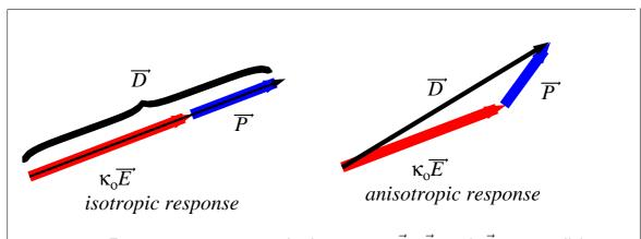
Figure 7-3: For an isotropic material, the vectors  $\vec{E}$ ,  $\vec{P}$ , and  $\vec{D}$  are parallel; in an anisotropic material the ions or electron clouds may be constrained to move in particular directions due to the underlying lattice or symmetry.
