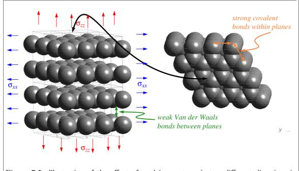
Figure 7-5: Illustration of the effect of applying a stress in two different directions in graphite. Because the deformation will depend on the direction that a particular stress is applied, the elasticity properties will be anisotropic.
