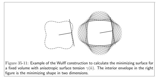
The Wulff construction is performed as follows:<sup>37</sup>
