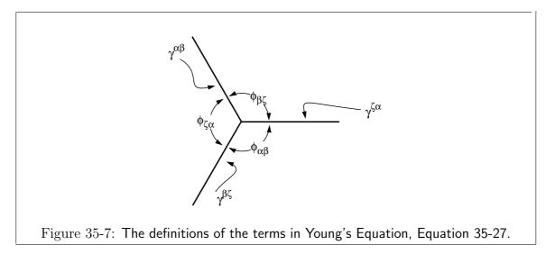
which is equivalent to the "force balance" where each of the  $\gamma$  are considered the forces applied to the vertex.
