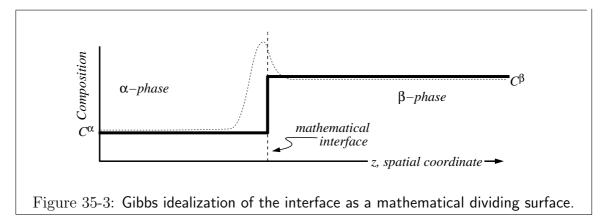
Subtract the real system in Figure 35-2 from its idealization in Figure 35-3 to define an excess quantity associated with the mathematical surface "The Gibbs Surface" which has no volume associated with it, but excess extensive quantities.
