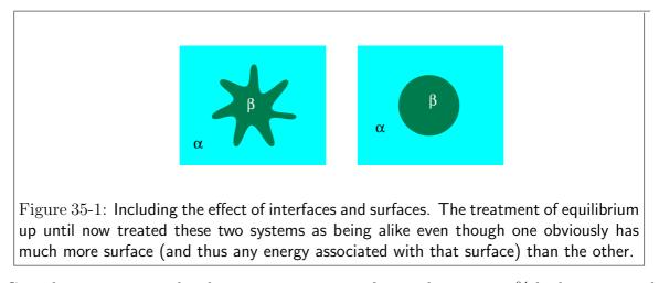
Consider, as an example, that an atom on a surface as having a 50% higher energy than those in the bulk, then there will be an extra energy associated with the surface of a sphere.
