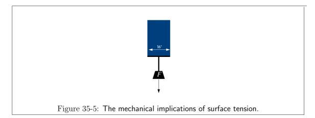
This is the surface tension, it has units of force per unit length or, equivalently, surface energy per area. It is the energy associated with creating surface.<sup>36</sup>
