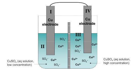
As in a standard Daniell cell, the membrane between the two aqueous solutions II and III allows only sulfate ions to pass.
