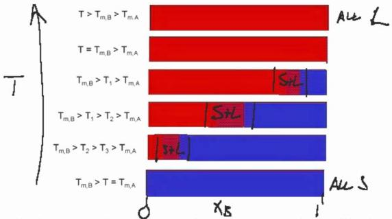
It would make sense to obtain a continuous map of the phases present as a function of X<sub>B</sub> and temperature for a binary system: such a map is a key tool in materials science & engineering and is known as a binary phase diagram. For the ideal binary solution we have been analyzing, the phase diagram looks like this:
