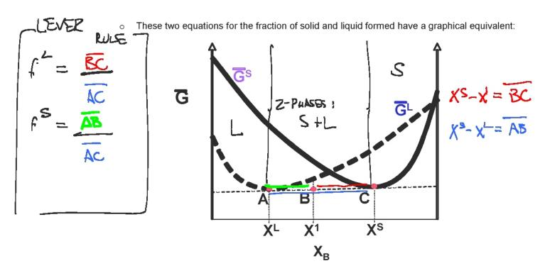
The mathematical and graphical construction to identify the fraction of each phase is known as the *lever rule*.
