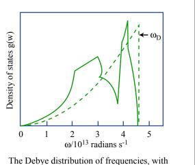
The Debye distribution of frequencies, with the experimental distribution of frequencies for copper. The distribution is shown as a function of  $\omega = 2\pi v$ . The experimental distribution is obviously complicated enough that a theory to reproduce such a distribution would likely be difficult to produce.
