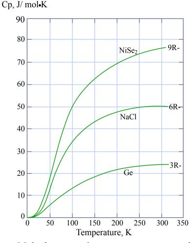
Molar heat capacity at constant pressure of three crystalline nonmetals.
