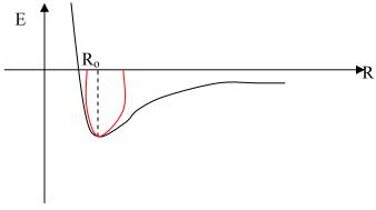
Figure 2. Schematic drawing of an energy-position plot for a diatom molecule. R represents the distance between the atoms. As shown from the red line near the equilibrium position ( $R_o$ ) the energy barrier can always be approximated by a parabola and thus the bond can be treated like a spring.
