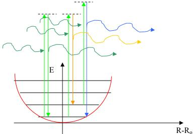
Figure 4 Schematic drawing of the three possible off-resonance interactions between an electromagnetic wave and an molecule. In the case of Rayleigh scattering a photon gets absorbed and immediately reemitted without gaining or loosing energy (left). In the case of anti-Stokes scattering a photon excites a particle that is in the first vibrational state. The particles then decays in the second vibrational state loosing energy (rigth). The opposite happens in Stokes scattering. (middle)
