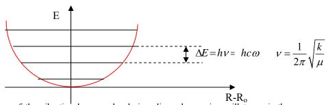
Figure 3 Distribution of the vibrational energy levels in a linear harmonic oscillator. v is the frequency expressed in  $s^{-1}$  while  $\omega$  is the wavenumber expressed in  $cm^{-1}$ .  $\mu$  is the effective mass, while k is the spring constant
