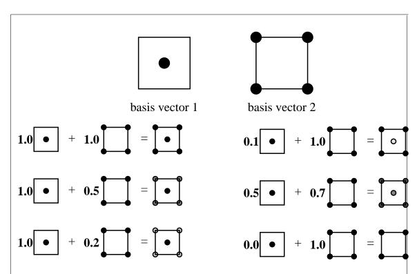
Figure 7-1: A vector space for two-dimensional CsCl structures. Any combination of center-site concentration and corner-site concentration can be represented by the sum of two basis vectors (or basis lattice). The set of all grey-grey patterns is a vector space of patterns.
