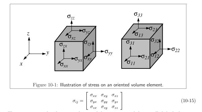
There is one special and very simple case of elastic stress, and that is called the hydrostatic stress. It is the case of pure pressure and there are no shear (off-diagonal) stresses (i.e., all  $\sigma_{ij} = 0$  for  $i \neq j$ , and  $\sigma_{11} = \sigma_{22} = \sigma_{33}$ ). An equilibrium system composed of a body in a fluid environment is always in hydrostatic stress:
