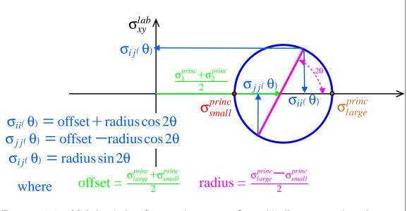
Figure 10-3: Mohr's circle of stress is a way of graphically representing the twodimensional stresses of identical stress states, but in rotated laboratory frames. The center of the circle is displaced from the origin by a distance equal to the average of the principal stresses (or average of the eigenvalues of the stress tensor). The maximum and minimum stresses are the eigenvalues—and they define the diameter in the principal  $\theta = 0$  frame.
