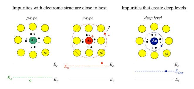
Impurity levels with respect to bands in Si, Ge and GaAs (typical semiconductors).
