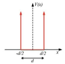
Consider the above system with the piecewise potential energy function V(x) for an electron inside the infinite potential well.
