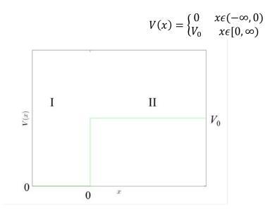
Find the general form of the wave functions for this potential energy and the transmission and reflections coefficients for the incident electron, R and T.
