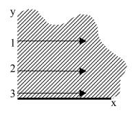
Three lines are shown on the object: 1, 2, and 3. Draw the temperature profile along each of these three lines, using one of the graphs below for each. Please draw profiles for an early time, at least one later time, and also for the steady-state. Also, next to each graph, write one brief sentence that explains your thoughts in making the graph.
