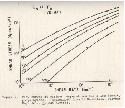
**Part B)** As a process designer, you would like to operate at the lowest possible temperature and the highest possible rate. Explain briefly how, with the help of this data, you would identify an optimum processing condition? What data would you need to do such an analysis?
