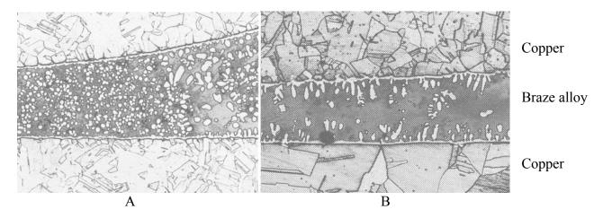
The process of brazing is essentially like casting: a melt is placed between two objects to be joined; the melt then solidifies, holding the objects together. These pictures show cross-sections of braze joints between two copper pieces (which are on the top and bottom).
