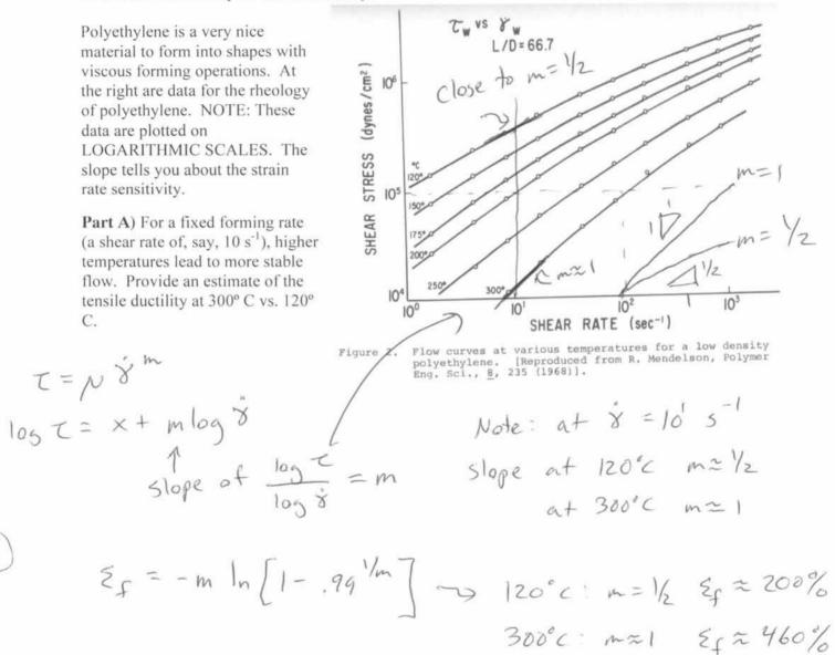
**Part B)** As a process designer, you would like to operate at the lowest possible temperature and the highest possible rate. Explain briefly how, with the help of this data, you would identify an optimum processing condition? What data would you need to do such an analysis?
