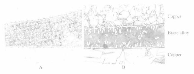
The process of brazing is essentially like casting: a melt is placed between two objects to be joined; the melt then solidifies, holding the objects together. These pictures show cross-sections of braze joints between two copper pieces (which are on the top and bottom).
