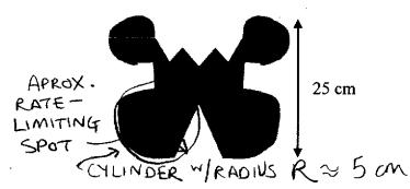
In the heat treatment of this shape, we need the whole piece to achieve a temperature between  $600^{\circ}$  and  $625^{\circ}$  C for 2 hours.
