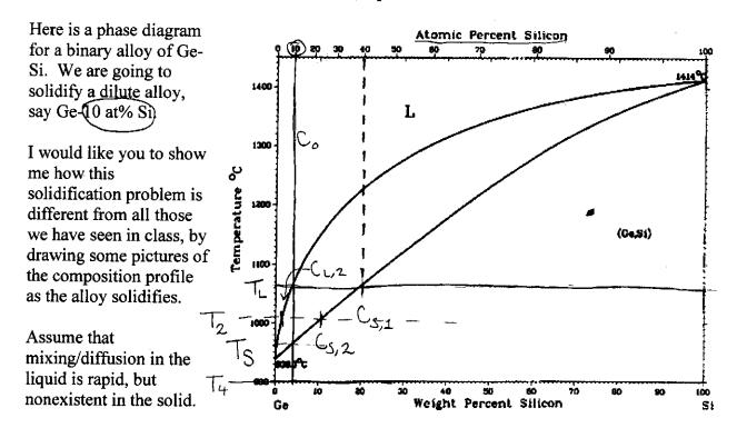
Please draw three pictures of the composition profile, at at least three times/temperatures. One near the beginning of the solidification ( $T = T_1$  near the liquidus), one at an intermediate time ( $T = T_2$ ), and one near the end of solidification ( $T = T_3$  near the solidus). Please make your charts as QUANTITATIVE as possible; label every quantity you can.
