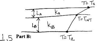
THE TOP SURFACE IS FIXED AT TI THE BOTTOM SURFACE IS FIXED AT TZ. THE 2 MATERIALS HAVE DIFFERENT THICKNESSES (LA, LB) AND THERMAL CONDUCTIVITIES (KA, KO) AND WE ASSUME NO INTERFACE
