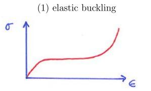
• buckling of vertical struts throughout honeycomb
