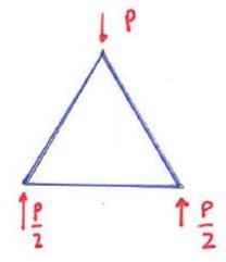
$$\sigma \propto \frac{P}{l b} \qquad \epsilon \propto \frac{\delta}{l} \qquad \delta \propto \frac{P l}{A E_s} \text{-axial shortening: Hooke's law}$$
