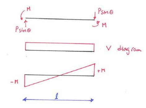
M diagram: 2 cantilevers of length l/2
