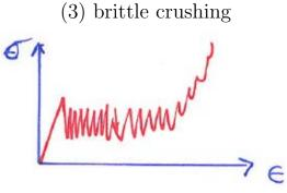
• peaks and valleys correspond to fracture of individual cell walls
