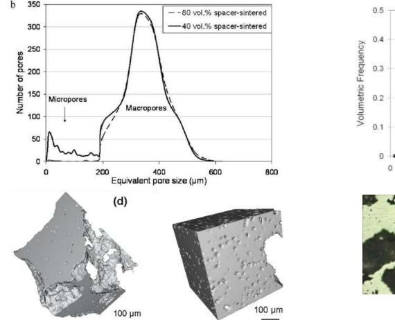
3D rendering of the pore wall<br/>parts of the foams produced<br/>with **80 vol. %** spacer.3D rendering of the pore wall<br/>parts of the foams produced<br/>with **40 vol. %** spacer.
