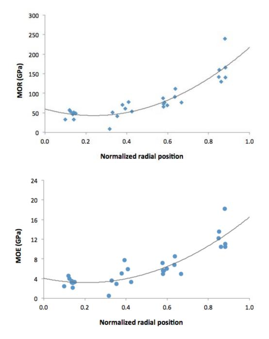
**Figure 4.8** *Top:* Flexural strength of Tre Gai bamboo with varying normalized radial position, *r/a. Bottom:* Elastic moduli with varying normalized radial position.
