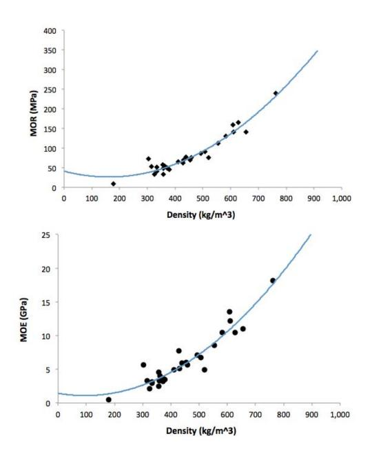
**Figure 4.7** *Top:* Flexural strength of Tre Gai bamboo with varying density. *Bottom:* Elastic moduli with varying density.
