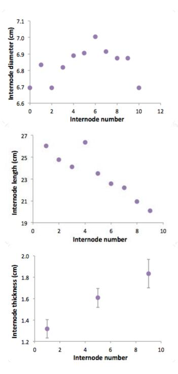
**Figure 3.2** Internode diameter (top), length (middle), and thickness (bottom) with varying internode number.
