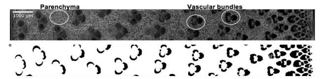
**Figure 4.1** *Top:* Tre Gai bamboo structure in cross section of the first internode. *Bottom:* binary-processed image of cross section
