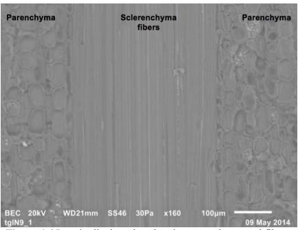
Figure 4.6 Longitudinal section showing parenchyma and fibers.
