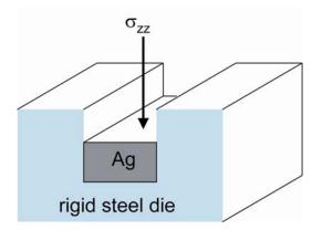
(a) Determine the orthogonal normal stresses in terms of applied stress and appropriate elastic constants of the material. Here, note that there are constrained and free surfaces created by the geometry of the die, such that the applied stress is uniaxial but the stress state in the material is more complex.
