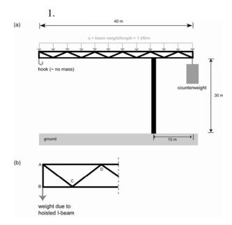
(a) Draw a free body diagram of the horizontal element of the crane (the horizontal span in Fig. 1a), treating it as a beam and indicating all known and unknown applied / reaction forces. You will need to make assumptions about how the crane is connected to the real world, and these should be briefly justified.
