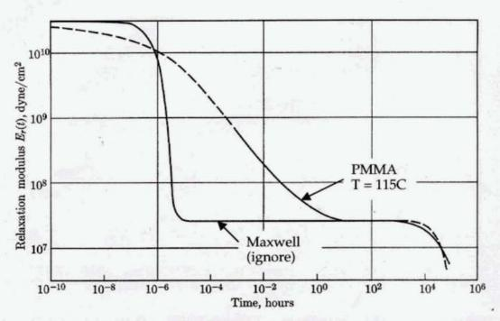
Fig. 6.25. Comparison of double Maxwell model with relaxation behavior of PMMA at 115°C, from Fig. 6.24.
