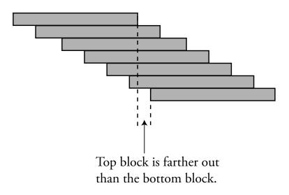
Figure 3: Collective center of mass of upper blocks is always over the base block.
