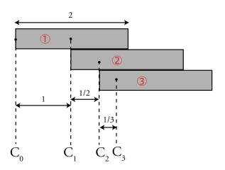
Figure 5: Stack of 3 Blocks. Left end of block 3 is  $C_2 =$  center of mass of blocks 1 and 2.
