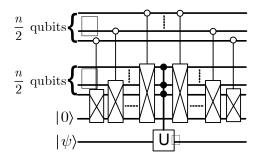
where the Fredkin gate with reverse polarity swaps the two input states if the control qubit is  $|0\rangle$  and does nothing if it is  $|1\rangle$ .
