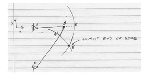
Augorithm to find B'1. If we only have  $u_x^B$ , what  $\delta^{AB}$  and  $\delta^{BC}$  would result? 2. If we only have  $u_y^B$ , what  $\delta^{AB}$  and  $\delta^{BC}$  would result? 3. What is the total  $\delta^{AB}$  and  $\delta^{BC}$  is I have both  $u_x^B$  and  $u_y^B$ ? for  $u_x^B$  and  $u_y^B$  from known  $\delta^{AB}$  and  $\delta^{BC}$ . Step 1
