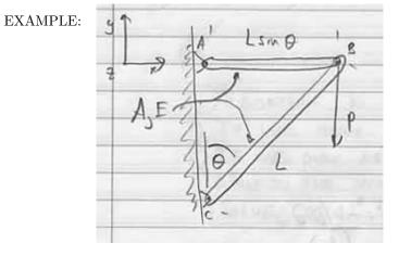
Q: Forces in bars? How much does each bar deform? How much does point B displace?
