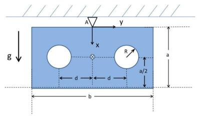
A pendulum consists of a rectangular plate (of thickness t) made of a material of density  $\rho$ , with two identical circular holes (of radius R). The pivot is at A.
