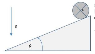
a) If the coefficients of static and kinetic friction between the wheel and the plane are  $\mu_s = 0.2$  and  $\mu_k = 0.15$  respectively, determine the maximum angle,  $\vartheta$ , of the inclined plane so that the wheel rolls without slipping.
